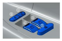
FIG.1 window control switch
