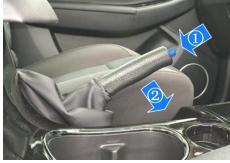
FIG. 60 release parking brake
