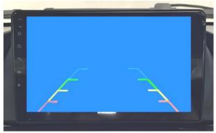
Fig 63 Display screen when reversing
