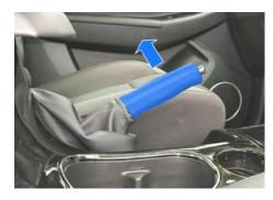
FIG. 59 Tighten parking brake
