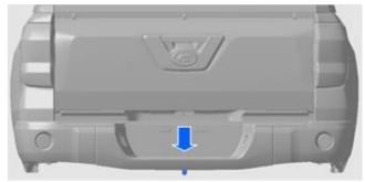
FIG. 62 Installation position of the reverse camera
