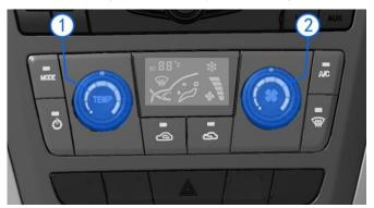
of the driver. The outlet temperature, blower speed (air volume) and air distribution can all be changed.
