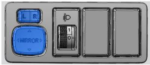
FIG. 28 Exterior rear-view mirror adjust switch
