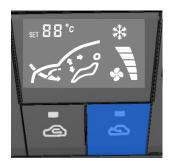
FIG. 49 Air external circulation switch
