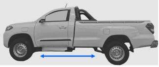
In order to ensure uniform wear of all wheels, it is recommended to periodically swap the left and right wheels of the vehicle at the same time according to the diagram shown in  $\Rightarrow$  Figure 91. This allows all tyres to have almost the same service life.
