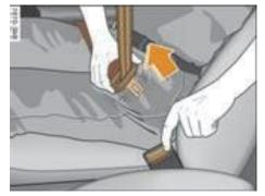
FIG.67 Release the latch from the seat belt latch
