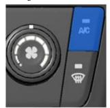
FIG. 50 A/C refrigeration switch
