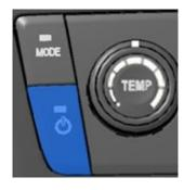
FIG. 39 A/C controller power switch
