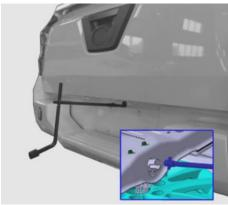
FIG.98 Remove and secure spare wheel
