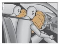
The airbag system is designed to trigger the driver and co-pilot airbags in the event of a more serious head-on crash.
