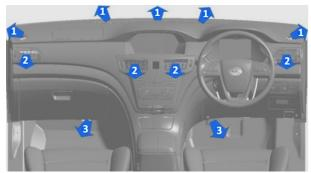
FIG.52 The position of the air outlet is arranged
