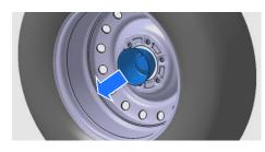
FIG.97 Remove the wheel trim cover
