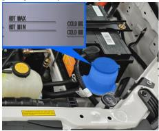
FIG.87: Marked position on the power steering tank
