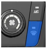
FIG. 51 Front defrost switch
