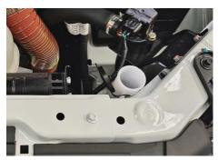
FIG.88 Open the window glass washing liquid storage tank
