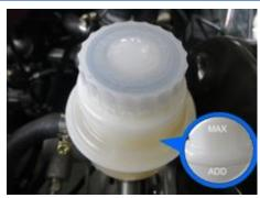
FIG.85: The mark on the brake fluid reservoir
