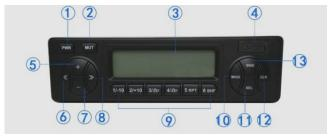
FIG.1 Control panel for the audio system
