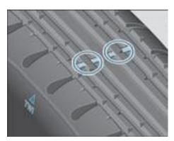
FIG. Tire pattern wear mark
