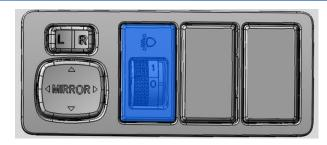
When the low beam of the vehicle is in the initial position, the position of the adjustment switch is 0.
